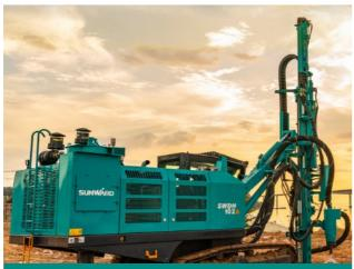
Paksehong Hydropower Station in Laos Basalt, 16-18, hole diameter D89mm, hole depth 15m, hole forming speed 13m/min, high temperature above 40°C, 18-24h continuous operation, challenger of high temperature and high strength.
