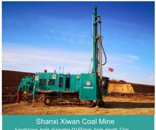
Sandstone, hole diameter D165mm, hole depth 17m, hole forming speed 50m/h, wet dust removal.
