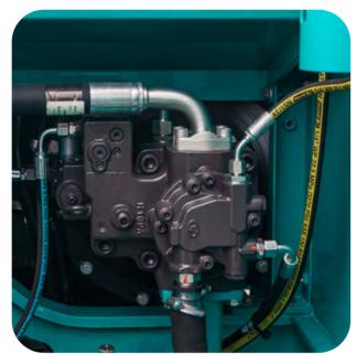
New electronically controlled variable main pump, combined with the large flow of the new generation of main valves, and the hydraulic system adopts a load-sensitive system which makes it more coordinated and more comfortable.
