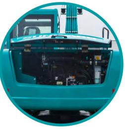
Neat and orderly upper vehicle arrangement, engine compartment is sealed to form an air duct.
